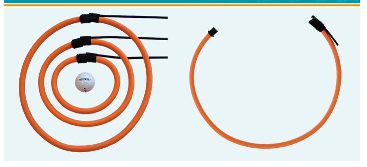
Accuenergy's Flexible Rogowski Coil is designed to use where regular solid or split core current transformers cannot fit, and ideal for power quality monitoring such as harmonics. Advantage including high accuracy, wide measruement and frequency range, and no additional integrator and power supply is needed.
